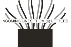
"J" boxes are utilized behind the wall to gather and consolidate incoming wiring from the individual letters. Depending on the LED capacity & size of letters, one box will accommodate six to ten letters. Multiple "J" boxes can be used for larger groupings of letters.
