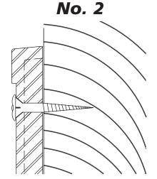
Wood walls flat head screws countersunk with rosettes
